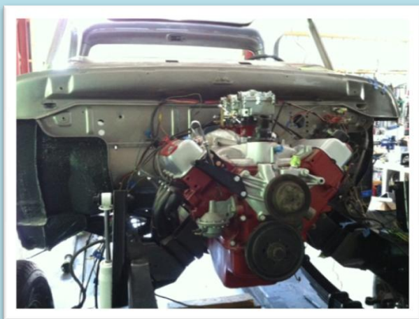
The poly head 318 installed in the truck after the rebuild
